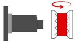
8. Next we place the outer spacer 9 on the upper machine shaft.
