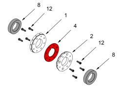
2. We do a pre-assembly, without tightening the bolts, paying special attention in aligning the slots for the pin.
