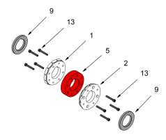
2. We do a pre-assembly, without tightening the bolts, paying special attention in aligning the slots for the pin.
