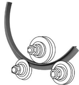
Adjustable rollers. The user may combine the set up position and it will allow bending the different profiles, adapting the sizes.
