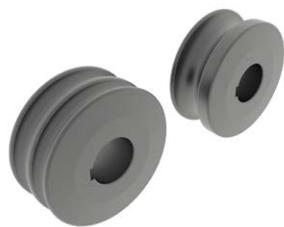
Rollers made of Steel F155 and treated to 62 Rc. Suitable for bending all kind of round steel or stainless steel pipes.
