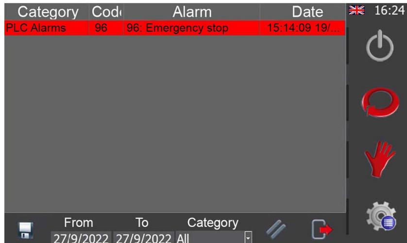
Here's a list of all the alarms that have gone off to date and all those which are still active are marked in red. To delete the alarms, they need to be corrected by unblocking the emergency stop button, for example. However, other alarms can be reset by simply pressing the
