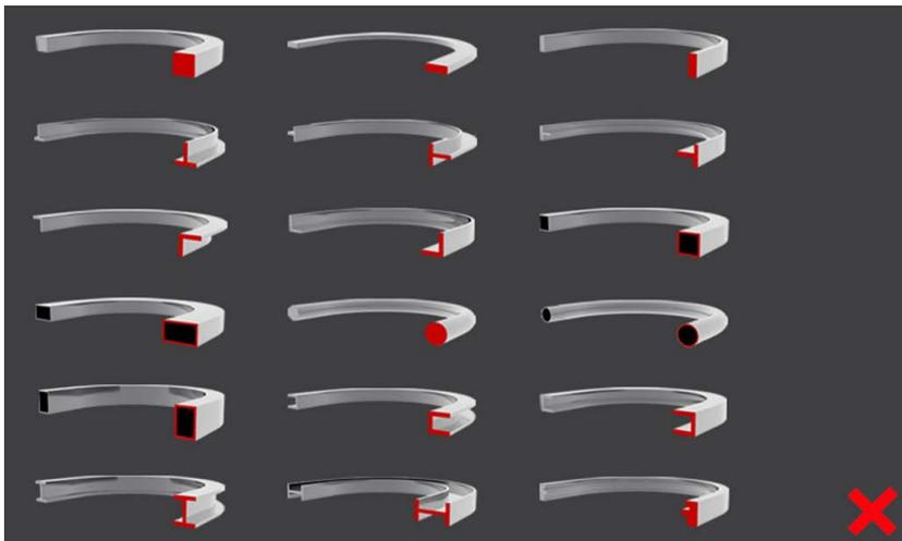
Remember the following data may vary based on the type of profile chosen. In other words, to define the dimensions when selecting a solid square profile, you must enter height and width. To define the dimensions when selecting a hollow square profile, however, you must enter height, width and thickness. Like-wise, you must enter the diameter if you choose round profiles.
