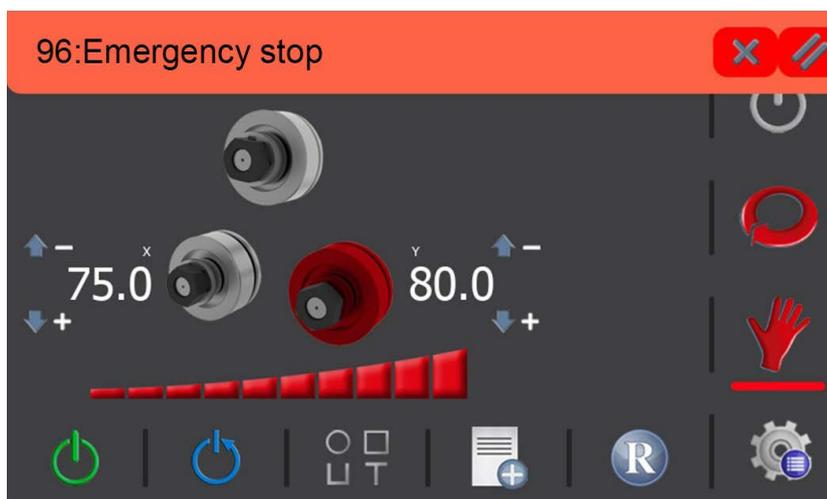
Remember that this window will also automatically close if the alarm disappears. In other words, in line with this example, this window will disappear if you unblock the safety button and press the reset button
