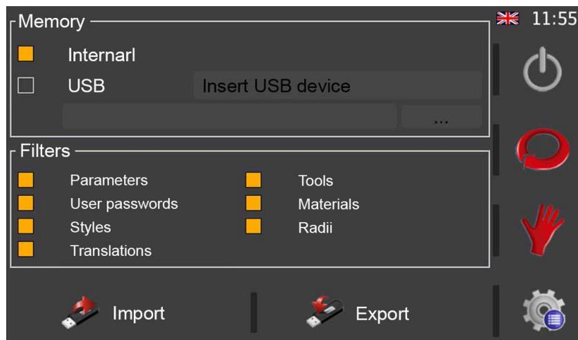
This screen allows you to export the data created on the PC and import them into the physical machine. Or vice versa. In other words, data can be exported from the machine and imported to the PC for the desired purpose if an operator has created new materials, tools or radiuses on the machine.
