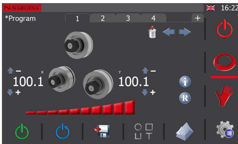
You can access any of the steps comprising the program by directly pressing the corresponding tab (the program is in step 1 in the image shown) or use the navigation arrows
