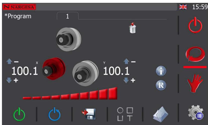
To access the automatic bender operating mode, just press the
