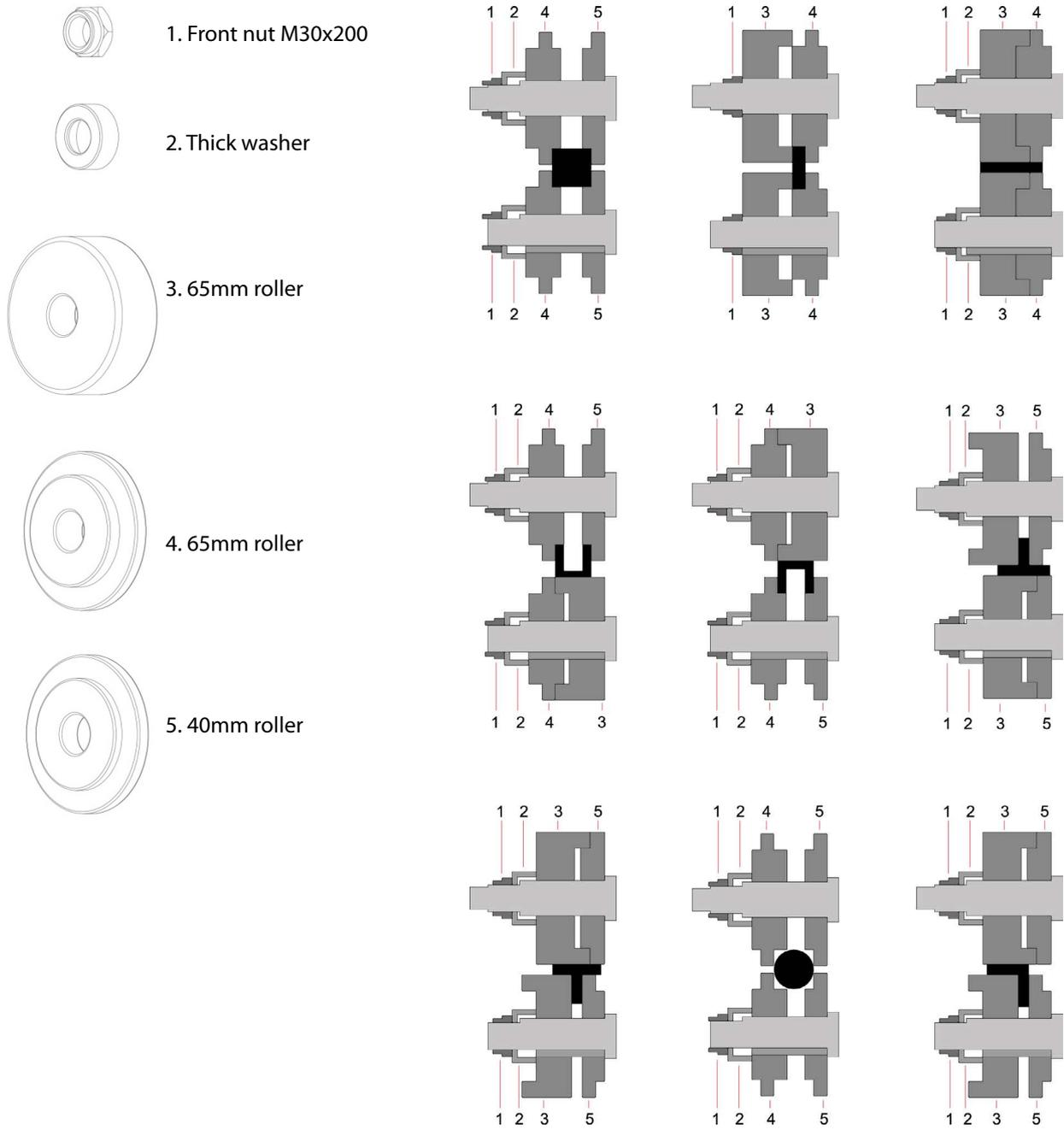
*Figure 14. Nomenclature of the rollers and assembly*
