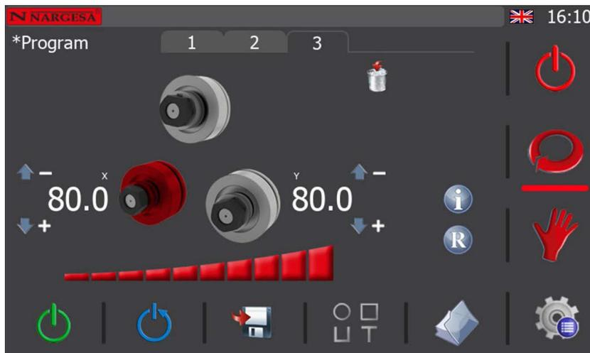
Upon doing so, the application creates a third step for the program. This step is known as the “clamping step”, which is when the material loaded in the machine and ready for processing is firmly secured between the upper roller and the two bottom rollers.
