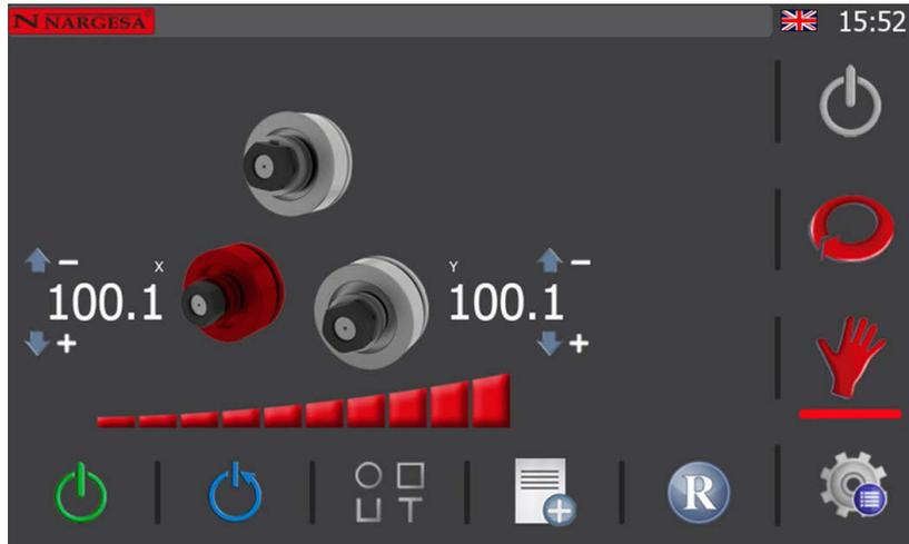
Now you can begin creating the sample bar. To do so, position each one of the rollers at a height so the profile to be worked can be loaded into the machine without any problems.
