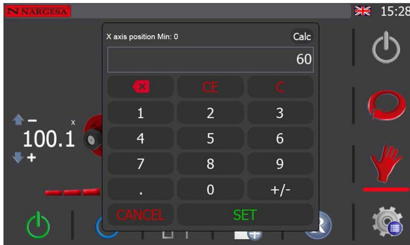
Enter the target height using the keypad. It's 60 in the example. Then, press the "SET" key on the screen to confirm and close the window.
