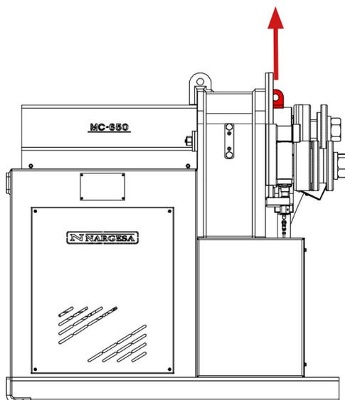
3. Lower it so that the part behind the machine bed is resting on the ground.
