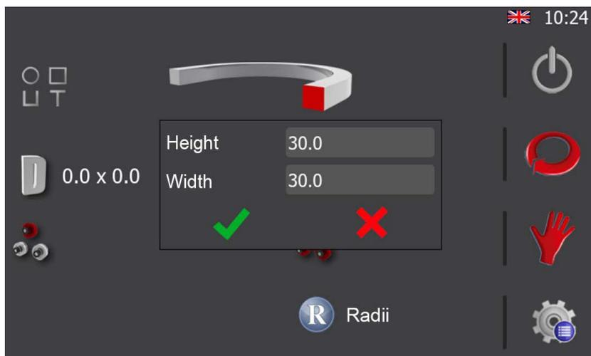
Once the profile dimensions have been defined to create the sample bar, select the material. To do so, press the
