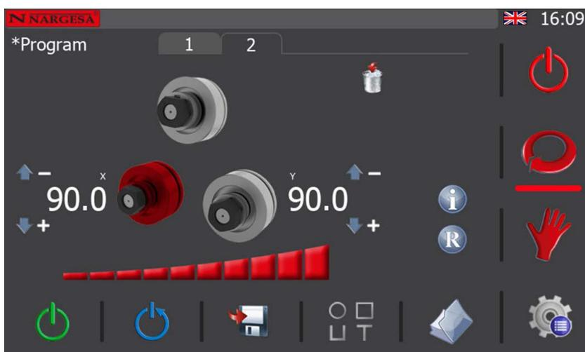
The second step in a program is known as the “loading step”. This is when the position of the bender rollers allows you to insert the material to be worked using the machine.
