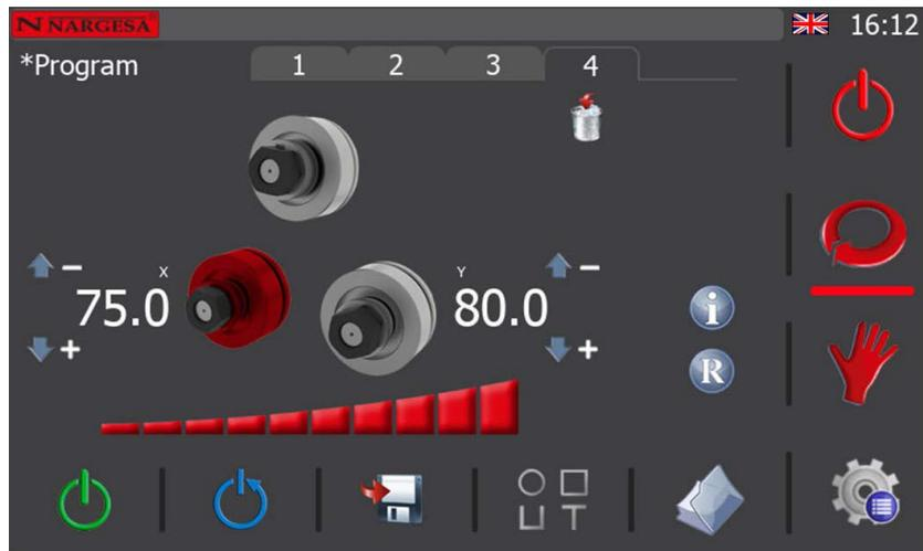
Now, with the material secured in the machine, it can be placed in position to begin bending by making the rollers rotate towards the left or right as learned in the section on the manual operating mode.
