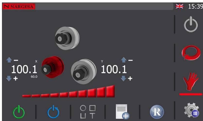
Now the machine is in the positioning mode for the X axis roller until the orange movement button located on the front of the control panel is pressed. Therefore, if you keep that button pressed down, the X axis roller will begin moving from the current height (100.1) to reach the target height established (60.0) at which time the positioning mode concludes (the target height on screen disappears).
