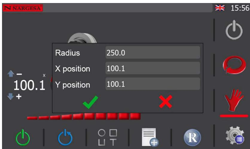
The position of the X and Y rollers will be captured automatically meaning the only thing you must now do is measure the radius by obtaining the first bend just created and enter that value in the “Radius” field in the prior image.
