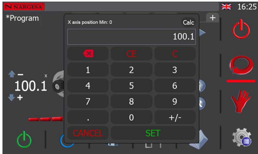
Use the numerical keyboard to make the adjustment to the height of the chosen axis. To confirm, press the “SET” key.
