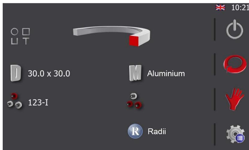
In the example, we have chosen a solid square profile. It appears at the top of the screen. Plus, we have assigned the dimensions 30.0 x 30.0. To do so, just press the
