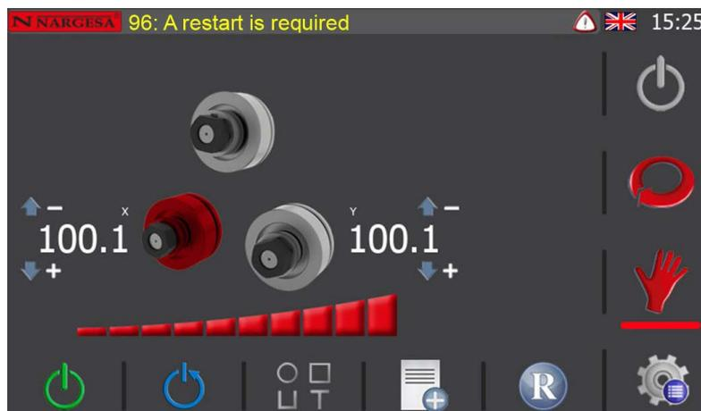
After turning on the power to the machine ("Power On"), the manual mode graphic interface is displayed on screen.
