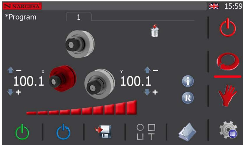
The first step in a program is known as the “unloading step”. As the name indicates, this is when the position of the rollers allows you to remove the piece created without it colliding with the rollers. Therefore, to create it, you just have to position the rollers on the X and Y axes at a height that will then make it possible to remove the finished piece once it is created.
