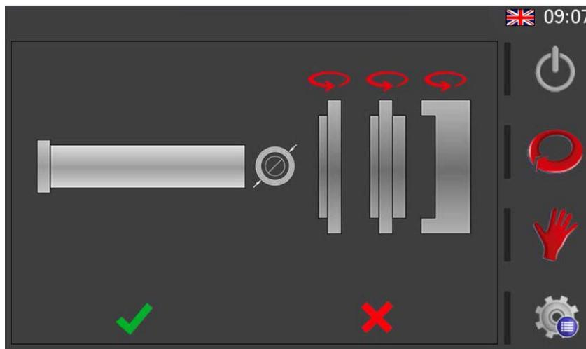
Using this interface, you can flip each one of the rollers (by pressing the arrow above them) and place them on the axis (by pressing the desired roller). Keep in mind that the order in which you press each one of the rollers will be the order in which they will be inserted on the axis.
