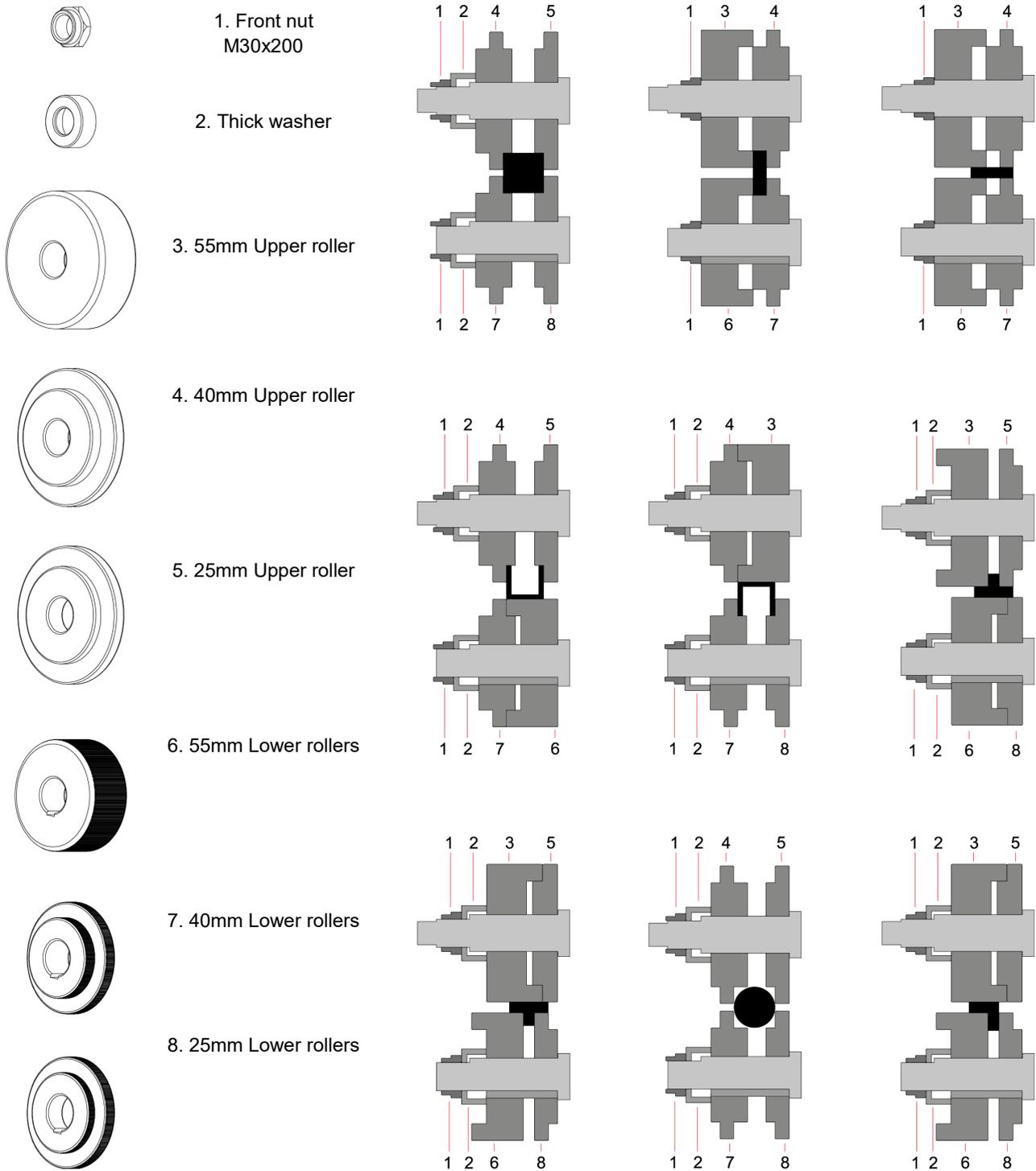
Figure 12. Nomenclature of the rollers and assembly
