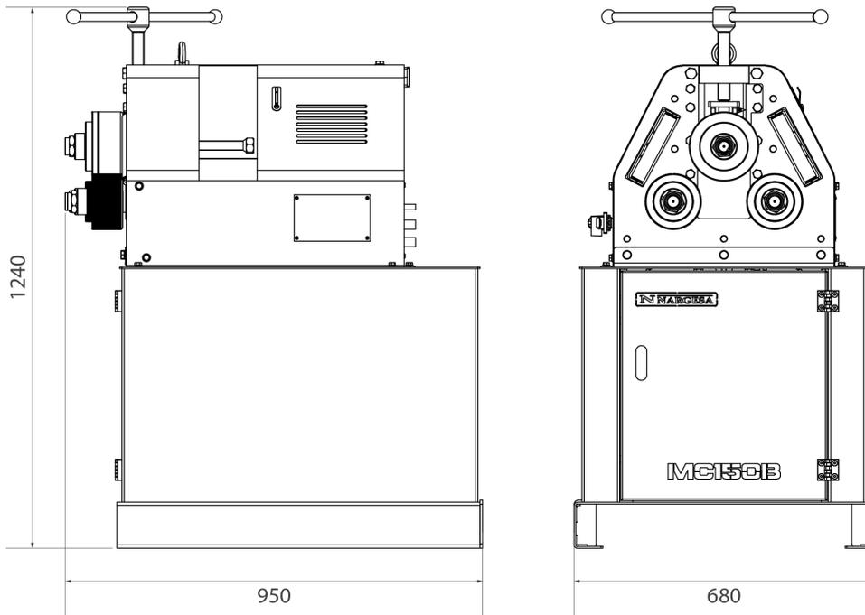
Figure 1. External dimensions of the MC150B bending machine
