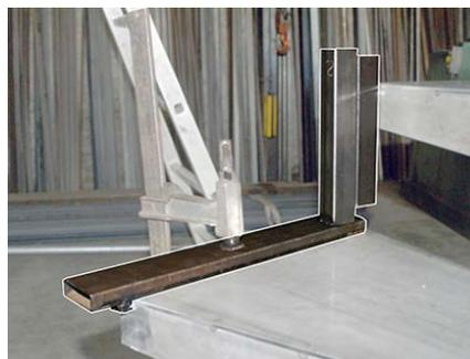
4. A special tool is anchored on the outside of the step. This makes stop at the front and side of the step and tells us where to put the next.
