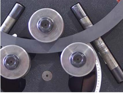
12. The MC400 Tube and Profile Roller is in charge of curving the handrail, giving it the exact shape without damaging it.
