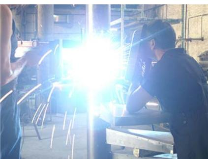
10. Proceed to permanently weld the step to the central tube. In this way we fix all the steps up to the proposed height.
