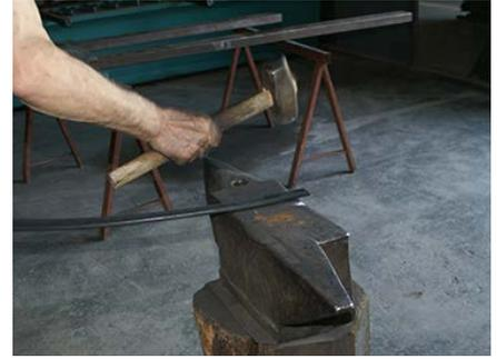
14. The handrail is twisted with a mallet to give it the perfect curvature.
