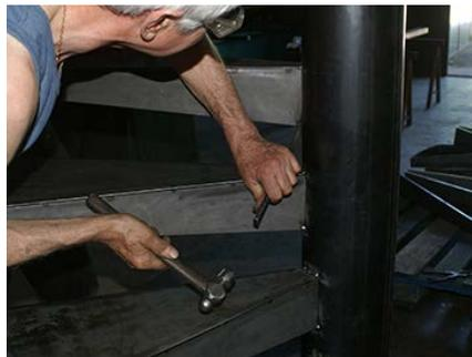
9. With smooth and controlled blows or small pieces of wire the deviation that may be corrected is corrected.
