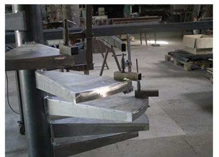
11. Next we have to manufacture the handrail of the spiral staircase. A tooling to which we mark the distance and the thickness of the handrail is fixed to the steps. These pieces allow to adjust the railing in an exact way.
