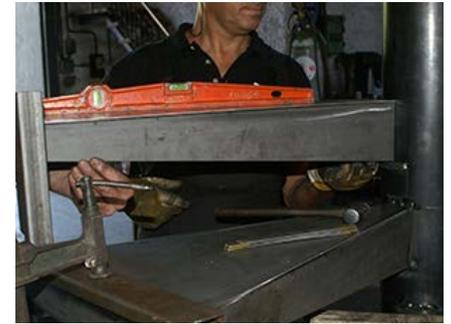
7. We level the step so that it is completely parallel to the ground.
