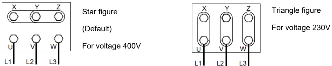
Picture 7. Change of engine connections
