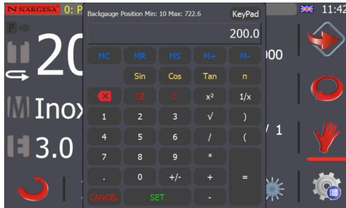
Once the required calculations have been done, the resulting value can be confirmed as the new cutting dimension by pressing the **SET** key.
