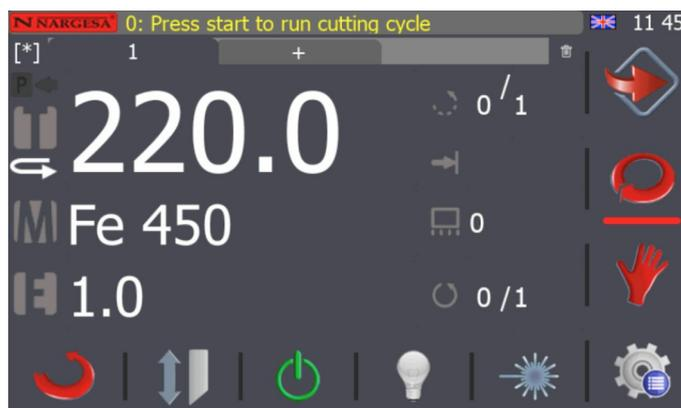
Automatic mode is similar to manual mode, with the option of specifying various operational steps with different cut dimensions. These specifications are saved within a program.
