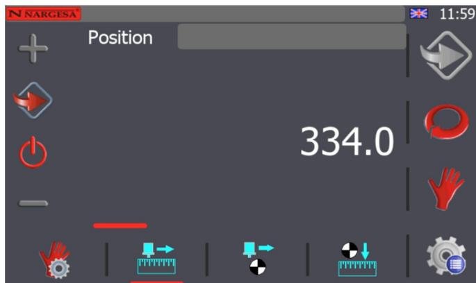
At this point, enter a value for the cut dimension that can be measured easily. 100 mm is a good option for example. Then, press the
