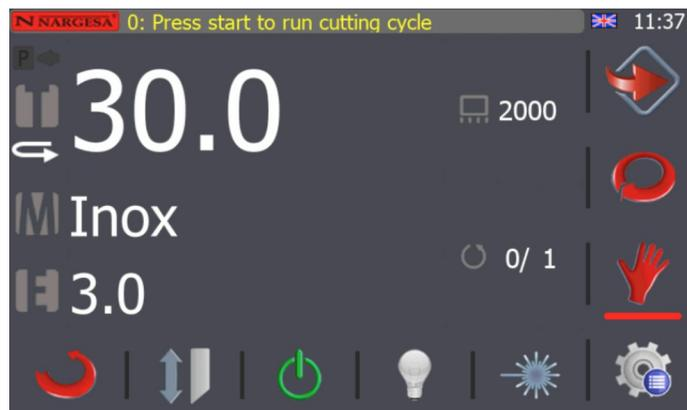
Cuts can be done manually from this point on by simply entering the information on the required cut. To input the cut measurements, press the corresponding button and the following screen will appear.
