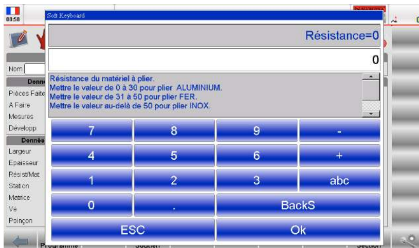
Figure 20. help page of the material resistance built-in the Soft Keyboard
