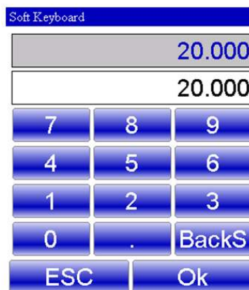
Figure 26 Soft Keyboard for setting the length of the piece
