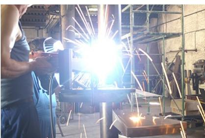
8. The step is fixed to the central tube with four welding points.
