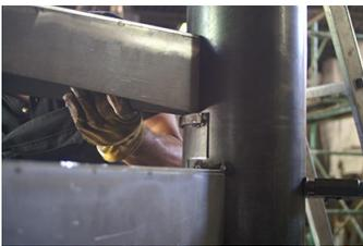
6. Place the step making stop on the tooling and the round bracket.
