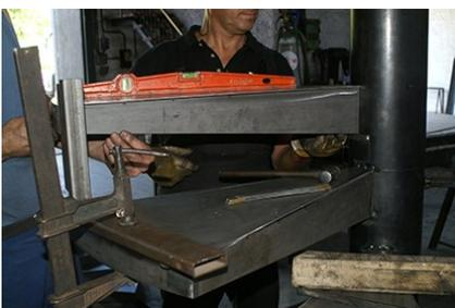
7. We level the step so that it is completely parallel to the ground.
