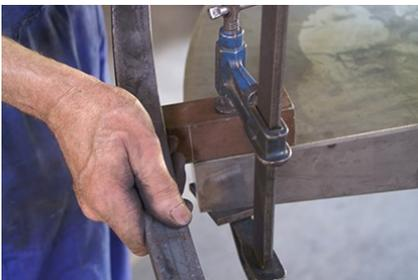
3. Check that the railing fits with the marks of the tooling.
