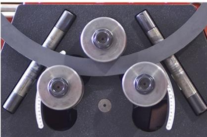
2. The MC400 Tube and Profile Roller is in charge of curving the handrail, giving it the exact shape without damaging it.
