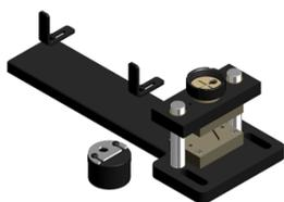
Tooling to flatten and punch the pipe for fences. It admits different pipe diameters. Exchangeable hole size.
