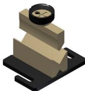
Tooling for folding sheet and flat bar up to 170mm. 88° punch. Dies with V for 56mm and V for 26m.
