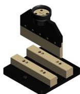
Tooling to fold metal sheet and flat bar up to 350mm. Punch: 88°. Die with adjustable V of 120mm, 80mm, 40mm and 16mm.
