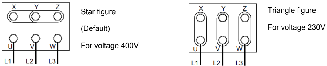
Picture 7. Change of engine connections
