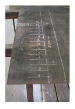
2. Draw a sketch on the scale of the elevation to check that at all times we have 220 cm between the overlapping rungs.
