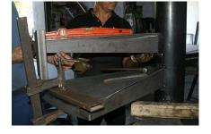
8. The step is fixed to the central tube with four welding points.
