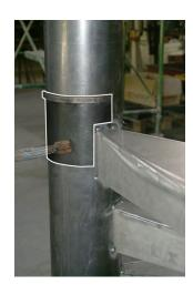
5. We use a round square made to measure that we fix to the tube, where the step will rest while we fix it.
