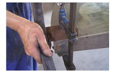
4. The handrail is twisted with a mallet to give it the perfect curvature.
