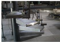
2. The MC400 Tube and Profile Roller is in charge of curving the handrail, giving it the exact shape without damaging it.
