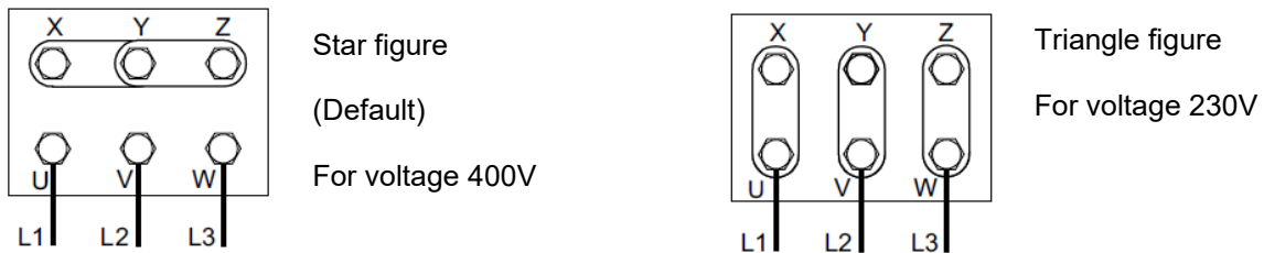
Picture 7. Change of engine connections
