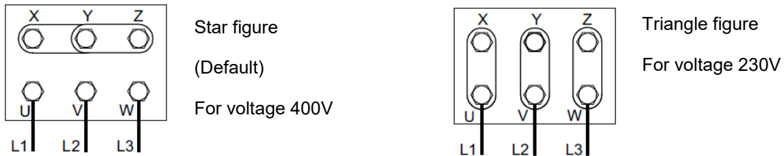
Picture 7. Change of engine connections
